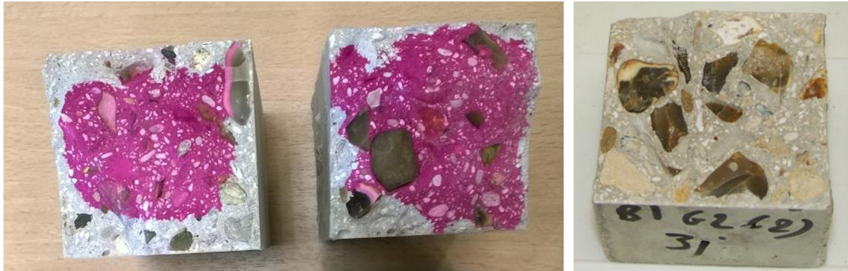
Figure 1.6. Views of split surfaces of specimens. Left: concrete B7 after phenolphthalein pulverization. Right: concrete B1 before phenolphthalein pulverization
