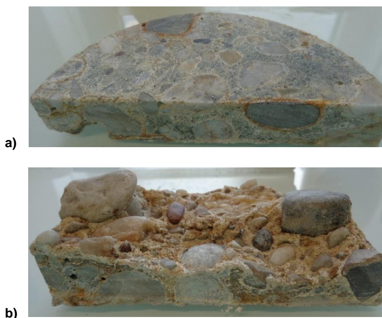
Figure 1.73. Photographs of CEM III/A concrete samples exposed for 4 months in the UGE biodeterioration chamber. Both samples are from a pumping station: a) sample from non-degraded area; b) sample from a degraded area
