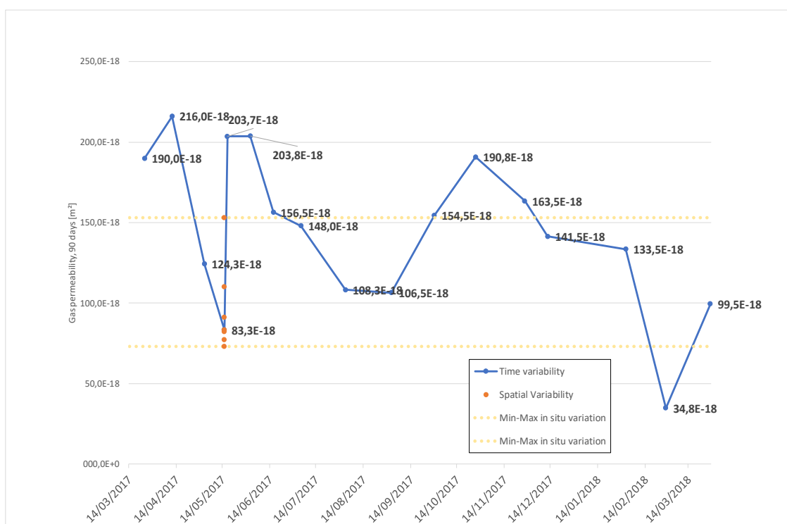
Figure 3.B.33. Gas permeability C40/50 viaduct La Reunion (temporal/in situ variability)
