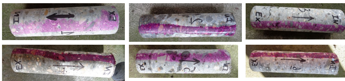
Figure 2.82. Lack of carbonation on all six cores
