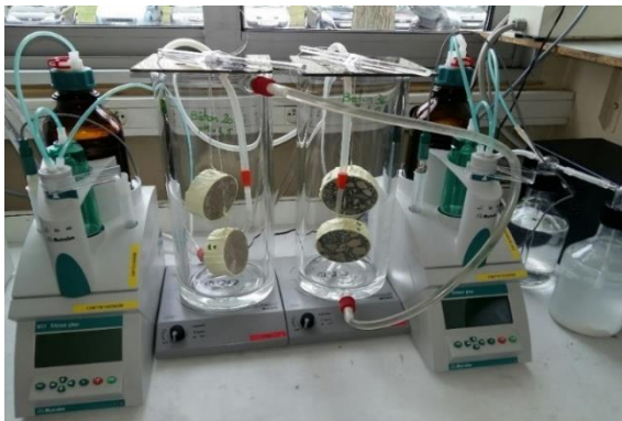
Figure 1.52 Picture of the set-up of the periodic leaching test
