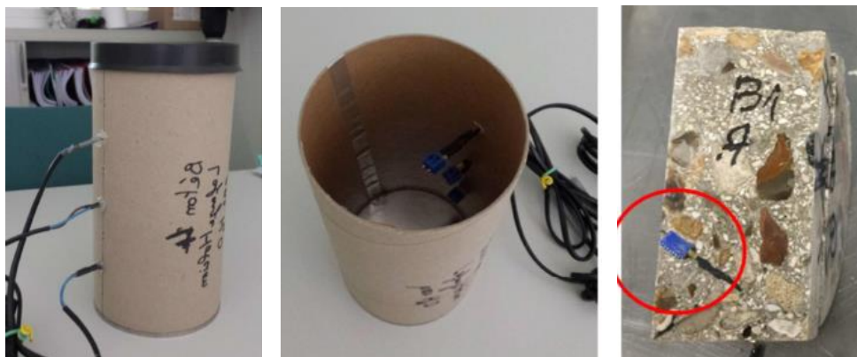
Figure 1.20. Device used for the monitoring of the water content inside a concrete specimen
